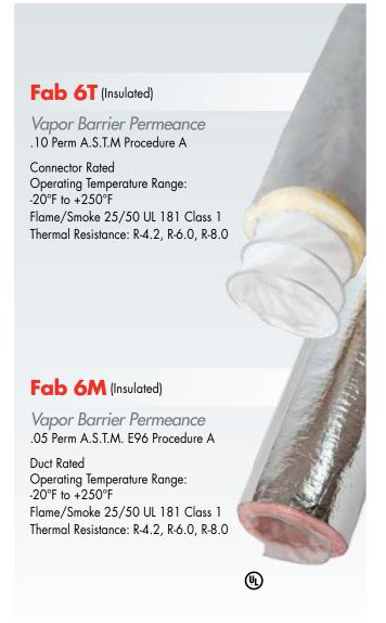
Flexmaster flexible ducting products are UL Approved as Class 1 Air Duct and have a Flame Spread Rating of not over 25 without evidence of continued progressive combustion and a Smoke Developed Rating of not over 50. Thermal resistance R4.2, R6 and R8.
