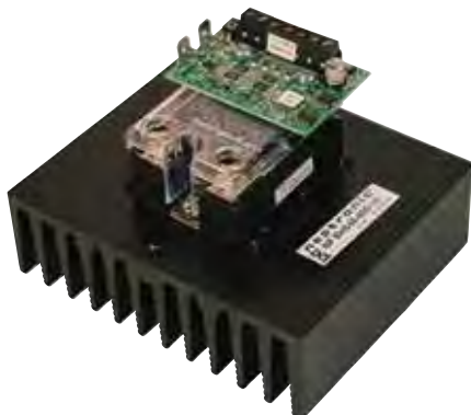
SCR Controller with SSR
